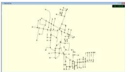
Fig:9: Chityala Village Network in EPANET
